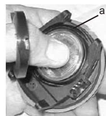
Fig. 137 - COVER & RING INSTALLATION
