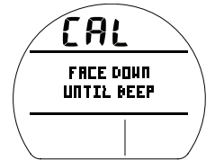
Fig. 121A - ACCESS TO CAL (turn unit upside down)
