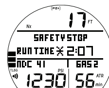
Fig. 50B - SS MAIN (set for Run Timer prior to dive)
