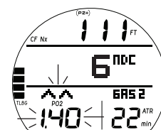
Fig. 64 - PO2 ALARM (during Audible)
