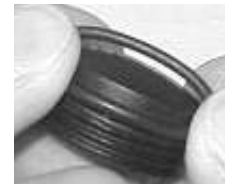
Fig. 142 - INSTALLING COVER O-RING
