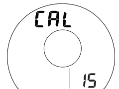
Fig. 123 - CAL PROGRESS (circle forms while rotating)
