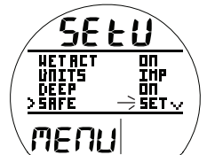
Fig. 26B - SET SS (to access Set Depth/Time)
