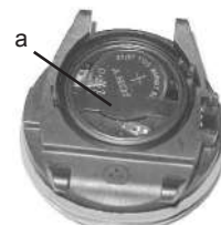
Fig. 136 - VT 4.0 BATTERY INSTALLED
