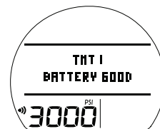
Fig. 2 - TMT BATTERY STATUS
